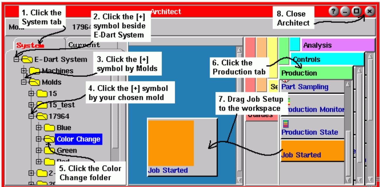
When purging the mold during a material change, stop the job and start the job with the “Color Change” folder. With the Job Started tool attached to that folder the *Job Started* output will go on. When running with the proper color (after the material change), stop the job and start the job with the correct color name.
