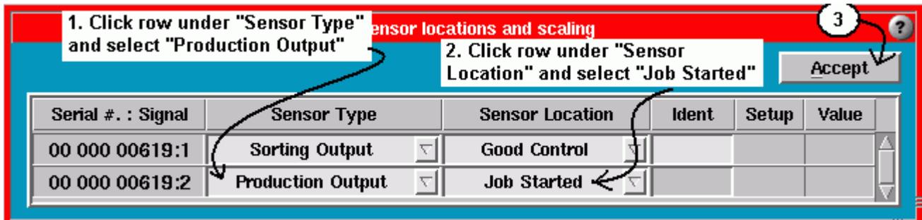
Note that the definition of the *Job Started* output remains with the machine. We assume that the contact closure is wired to the machine. Therefore regardless of which mold you run on the machine the output will remain defined as *Job Started*.
