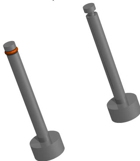
Figure 5: Example of a static pin with an O-ring. The O-ring helps minimize flashing around the flush mount sensor or the static pin
