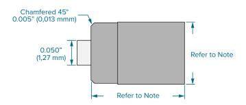
NOTE The sensor is press fit. Gauge each sensor body, then cut each sensor pocket. Once sensor is installed in mold, machine the sensor tip down to be flush with the cavity surface. The finished sensor length may not be less than 0.177" (4,496 mm). Refer to installation instructions and specifications in the product manual.
