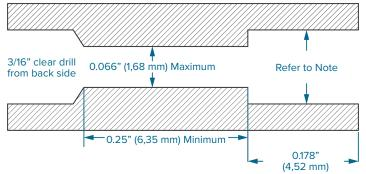
The wire channel maximum diameter of 0.066" (1,68 mm) is specified to ensure sensor body support under pressure. The channel does not need to be enlarged as shown.
