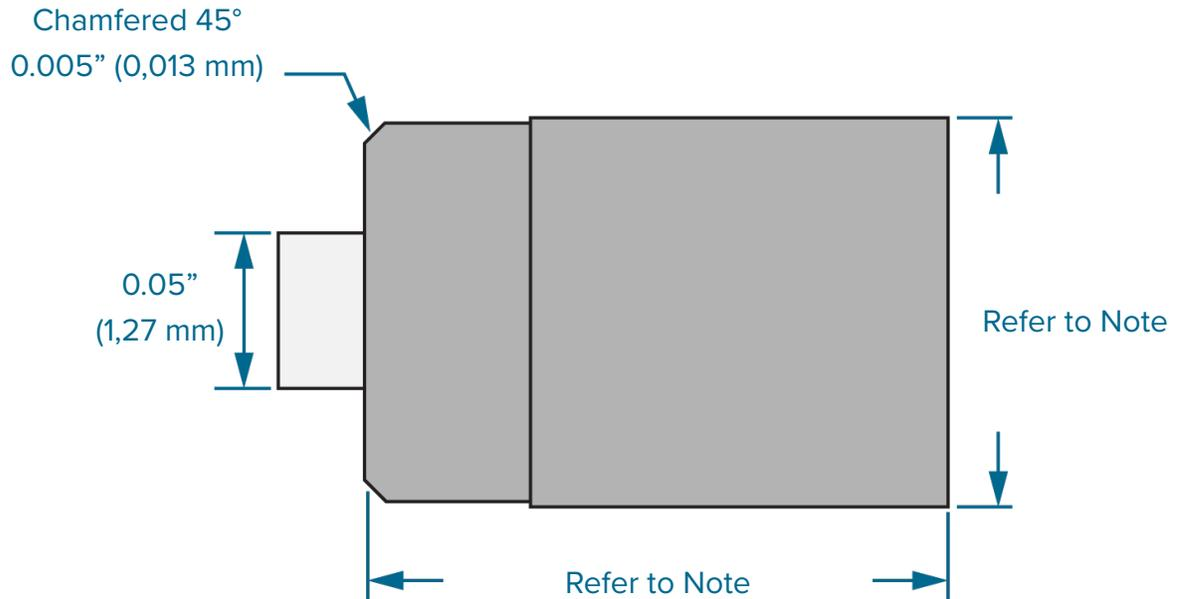
**NOTE** The sensor is press fit. Gauge each sensor body, then cut each sensor pocket diameter: Refer to “Sensor Head Pocket” on page 10.
