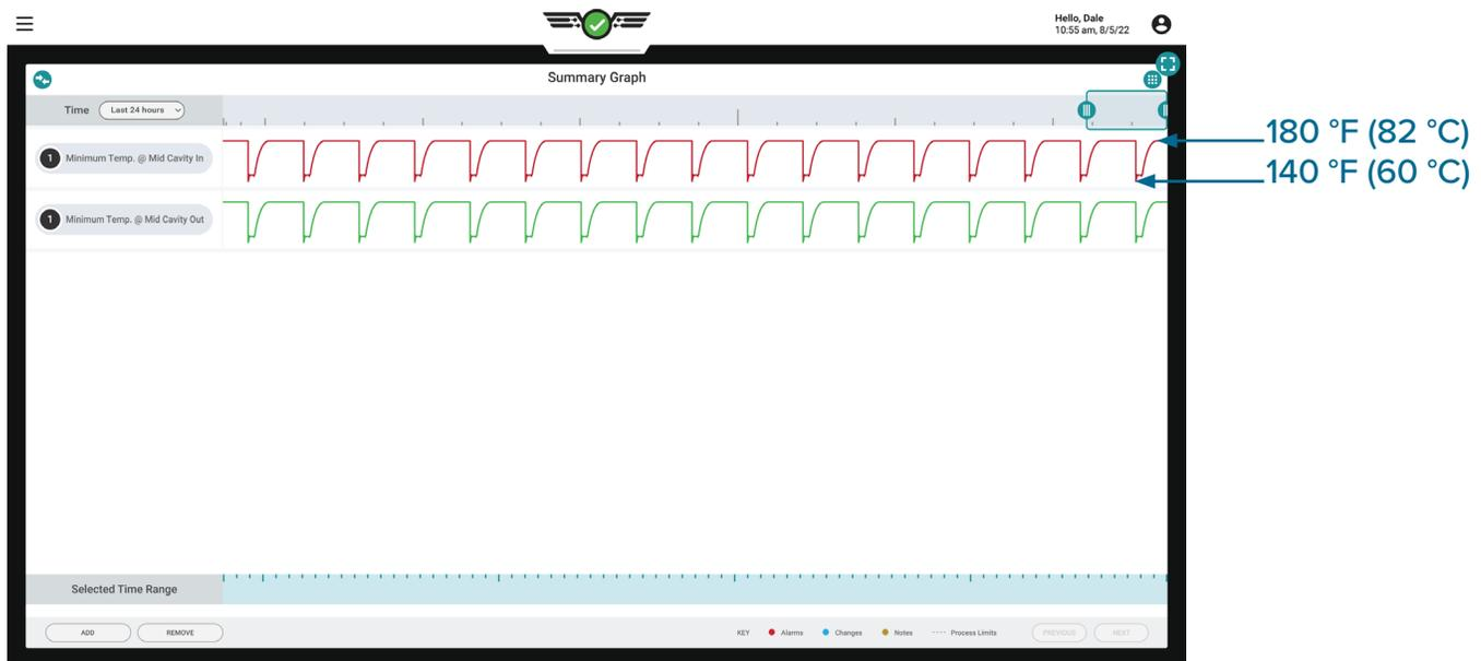
The time to reach stability is often longer than anticipated, so the concept of identifying mold temperature stability is important when preparing a process for “lights out” operation, or before parts are sampled for measurement.
