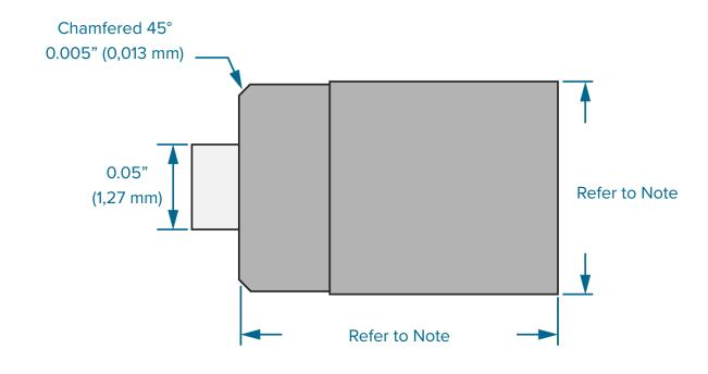
The sensor is press fit. Gauge each sensor body, then cut each sensor pocket diameter: **(i) NOTE** Refer to "Sensor Head Pocket" on page 10.
