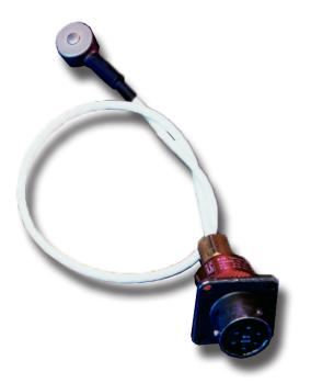
The analog single-channel strain gage sensor T-445 are indirect (under pin), 0.625" (15,88 mm) button-style cavity pressure sensors that can withstand forces up to 4,000 lb. (17,79 kN) and temperatures of up to 250 °F (121 °C—standard sensors) or 425 °F (218 °C—high-temperature sensors).
