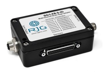
The Lynx™ eight-channel strain gage sensor adapter with mold ID SG/LX8-S-ID is an adapter that interfaces the RJG, Inc. Lynx™ eight-channel strain gage sensor connector SG-8 and up to eight multi-channel strain gage (MCSG) sensors to the eDART® or CoPilot® systems.
