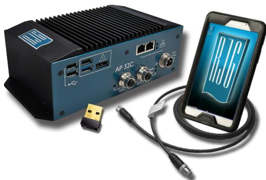
The Sensor eValuator provides testing of up to 30 Lynx™ cavity pressure sensors simultaneously, including the automatic testing of strain gage sensors for lynx communication, zero offset, and broken wire/failed gage tests; automatic testing of piezoelectric sensors for lynx communication and drift tests; manual testing of strain gage sensors for basic force detection; and manual testing of piezoelectric sensors for basic force detection.
