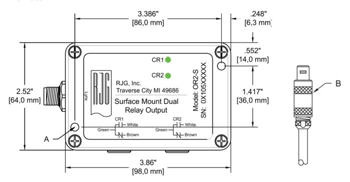
Figure 1: A. Drill and tap for 10-24 threads B. C-OR2/LX-4M
