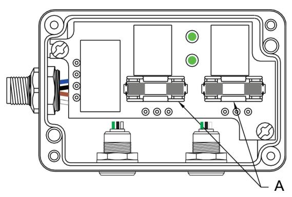
Figure 3: Relay Output Replaceable Fuse Location
