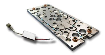
The LES-B-127-50/125/500/2000 are multi-channel, digital strain gage, indirect (under-pin) 0.50" (12,7 mm) button-style cavity pressure sensors designed for use with the RJG eDART® and CoPilot systems. One Lynx™ connector connects up to 16 sensors and to one system Lynx port (up to 32 sensors per system—additional sensors will require additional systems); if more than 32 sensors are required please contact RJG Customer Support for additional information.
