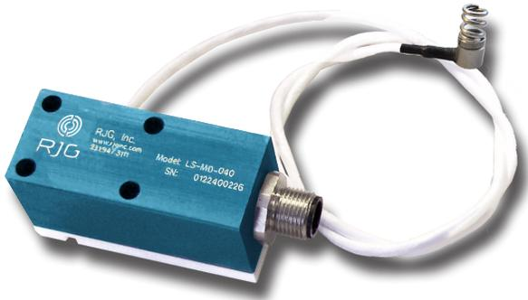
The Lynx mold deflection sensor LS-MD-040 measures up to 0.040" (1,016 mm) of mold deflection at the parting line each cycle for use with the eDART® system.
