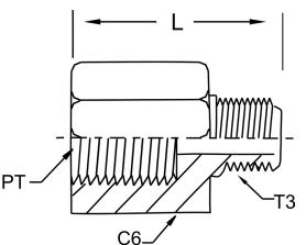
Figure 23: Conversion Adapter-BSPT NPTF dimension drawing
