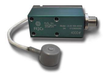
The LSB159-4000 is a single-channel, digital strain gage, indirect (under pin), 0.625" (15,88 mm) button-style cavity pressure sensor designed for use with the RJG eDART® or CoPilot® process control and monitoring systems.
