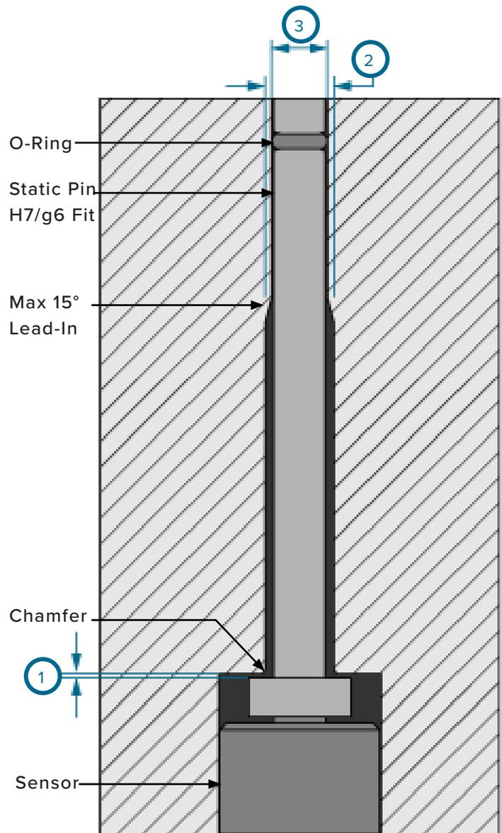
**CAUTION** These guidelines are for pins 3/32” (2,5 mm) diameter or larger. Please contact RJG Customer Support for installation of static pins smaller than 3/32” (2,5 mm) in diameter
