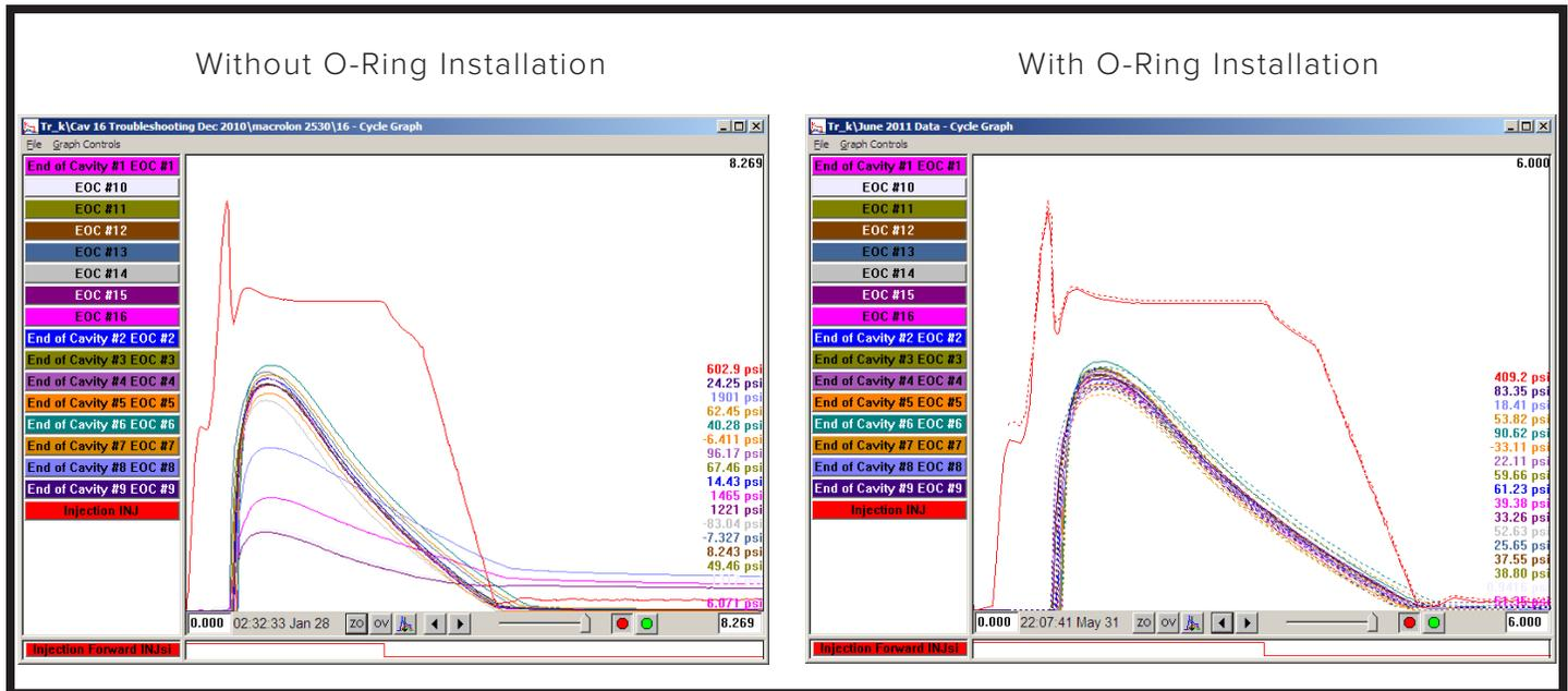
Above Left: Three sensors are reading too low due to contamination—without O-rings installed.
