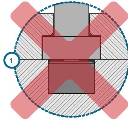
2. Sensor head is installed incorrectly (2 at right).
