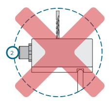
4. Orientation of Lynx connector on Lynx case is altered from OEM (3 at right).
