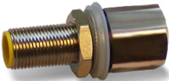
The Lynx™ Single Feed-Through Junction J-LX1 is installed on injection molding machines to connect machine interface DIN-rail modules mounted inside the machine panel to the eDART® or CoPilot® systems outside the machine panel.
