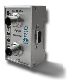
The Lynx™ shielded sequence module is a DIN-rail-mounted module that is wired to the molding machine in order to collect 24 V DC timing signals for use with the eDART® or CoPilot systems, including injection forward, screw run, mold closed, first stage, and mold opening. The use of an ID7-M-SEQ (or a DIN/LX-D) module is required to physically connect to the eDART system. This DIN-rail module is shielded to ensure high-quality data even in rugged molding environments.
