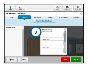
In the Coolant Flow Rate pop-up window, select the 4 VM-#-#-150-B sensor model from the Sensor Model drop-down menu. Select the 5 Location from the drop-down menu. Click the 6 Save button.
