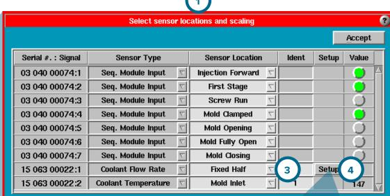
Click the drop-down menu in the Sensor Location column in line with the "Coolant Flow Rate" in the Sensor Type column to set the location.
