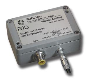
The Lynx™ surface-mount analog input module IA1-S-VI-24 is a surface-mounted module that is wired to the molding machine in order to collect 0–10 V DC or 4–20 mA signals from analog measurement devices, providing information such as injection pressure, plastic pressure, screw position, or temperature. This module can supply a 24 V power source to some sensors, and is shielded to ensure high-quality data even in rugged molding environments.
