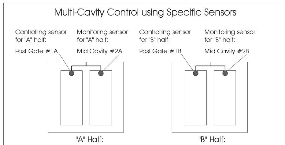
Setting control to “Post Gate #High” will control off of “Post Gate #1A” when in the “A” position and “Post Gate #1B” in the “B” position.
