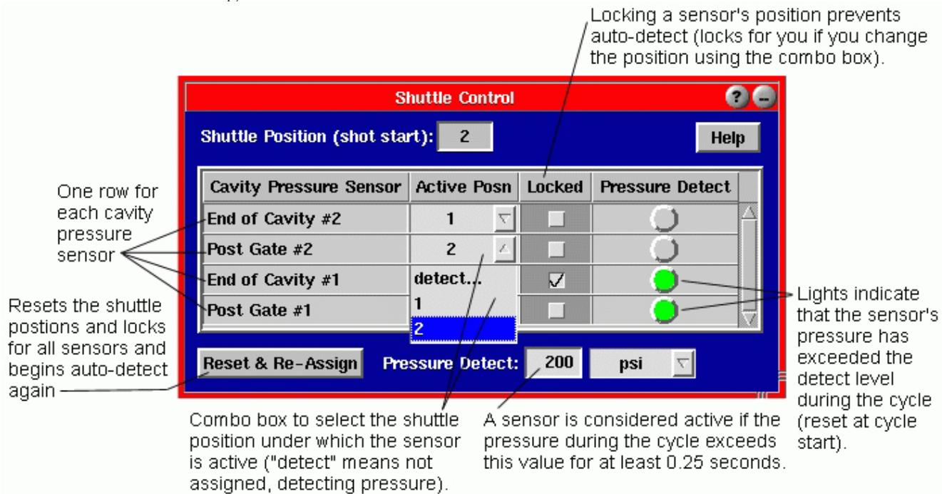
The Active Position column will show “detect” if pressure has not yet been seen on this sensor and the sensor is not yet assigned. The Shuttle Control tool will be looking for pressure. Also, if the position shows “All” it means that it is active in both positions “1” and “2”. The shuttle control will automatically set the value to “All” if it sees pressure over the threshold for longer than 0.25 seconds in both positions.
