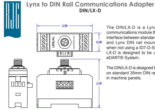
The DIN/LX-D is a Lynx to DIN rail communications module that acts as an interface between standard Lynx cables and Lynx DIN rail mounted modules when not using a ID7-D-SEQ. The DIN/ LX-D is designed to be used with the eDART® System.
