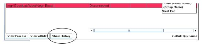
The **History** will show how a machine ran against its template values on ASO. Every cycle that ran optimally will have a **green** sliver added to the time line. rejects will show as **red** and suspect **yellow**. Many red slivers means a lot of adjustments (tweaking) were made, or that the machine is not capable of running a repeatable process – such as leaking checkring, bad hydraulic valves, etc.
