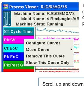
To add curves choose **Configure Curves** and click on the column on the left for **Types** of values and click on **Visible** column for the **Location** to display and click on **Color** (a color palette will appear) to apply to it.
