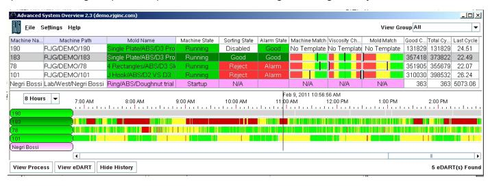
**Note**: For eDART<sup>™</sup>s with version 9.0, the **Process Stability Dashboard (PSD)** must be activated on the eDART<sup>™</sup> for the **Show History** to function.
