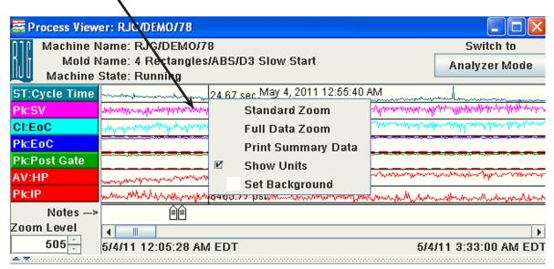
Right click in the Cycle Graph curves to adjust the Zoom, print cycle, show templates, overlays, adjust cursor display, reset scale or change background color.
