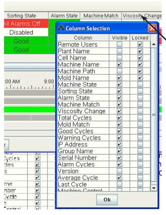
To customize your view on the EDM, right click on any column header to enable the Column Selection. Choose a value you would like to display on the ASO and put check mark on the box under Visible column.
