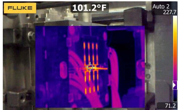
Image 3: Part Temperature at Ejection for ABS
