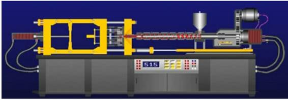
Figure 4: Toggle molding machine unsupported in the center of the moving half
