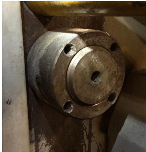
Image 2: Gap between platen and tie bar nut
