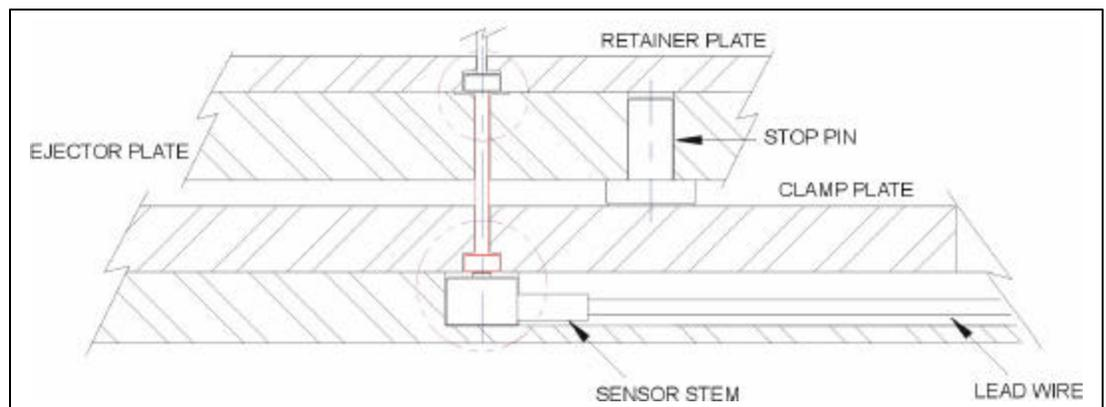
Figure 4: Indirect using a transfer pin
