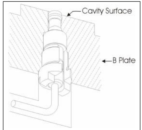
Figure 2: Flush Mount installation
