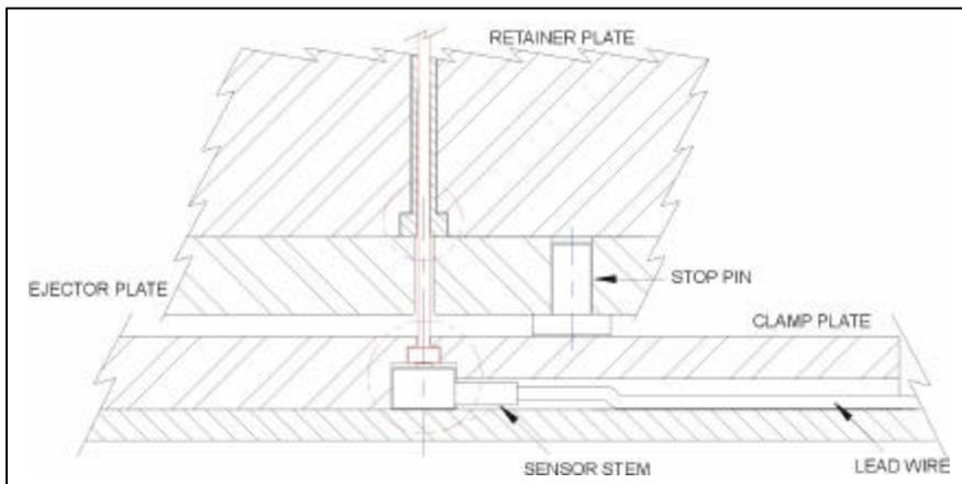
Figure 3: Indirect sensing through an ejector sleeve
